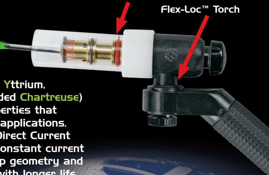
New LaYZr™ (1.5% Lanthanum, 0.08% Yttrium, 0.08% Zirconium) Tungsten, (color-coded Chartreuse) is non-radioactive and has great properties that make it best at automated or robotic applications. LaYZr™ can be run in Alternating or Direct Current using inverter or transformer based constant current power sources. It has a very stable tip geometry and runs 30% cooler than 2% Thoriated, with longer life.
